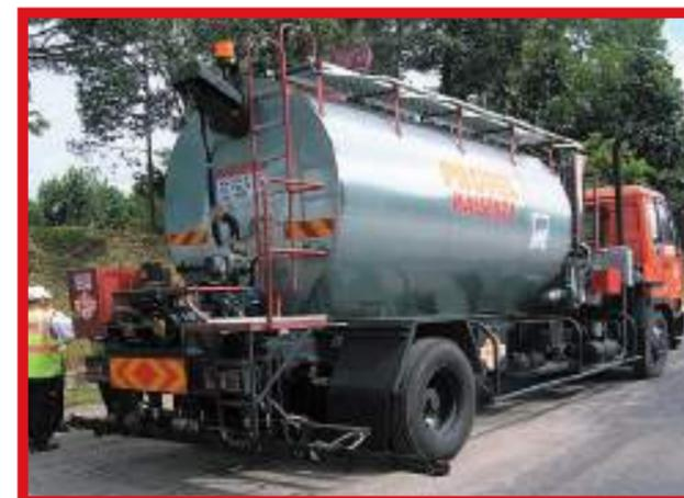
Design and construction of specific spraying tank model suitable for neat bitumen or Polymer Modified Bitumen (PMB), including all the most advanced technical solutions required to ensure a trouble-free use of these high viscosity products.
