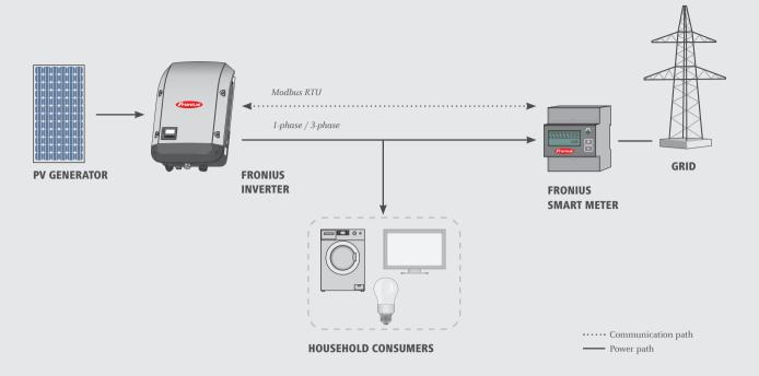
/ The Fronius Smart Meter is compatible with all inverters with an RS485 interface (Modbus RTU). The Fronius Smart Meter works in conjunction with the Fronius Datamanager 2.0 for the Fronius IG¹), Fronius IG Plus and Fronius CL inverters, whereas the Fronius Datamanager Box 2.0 is used with the Fronius IG TL, Fronius Agilo and Fronius Agilo TL inverters. The Fronius Smart Meter can be retrofitted at any time together with the Fronius Datamanager 2.0 in inverters that have already been installed.
